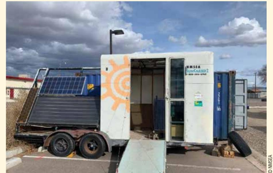
The original SunChaser was built on a flatbed trailer, housing a small enclosure as well as an exterior PV rack.
